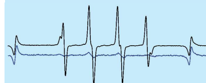
Fig. 1 ESR Spectra of hydroxy radical adduct
